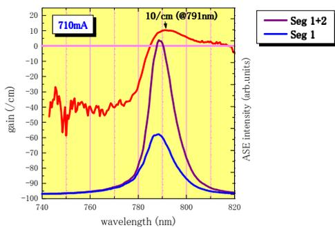
**Fig.1** Amplified spontaneous spectra (ASE) when single 500- $\mu\text{m}$ -long stripe (Seg 1) or double stripes (Seg 1+2) were excited. Modal gain spectrum is deduced from the two ASE spectra.
