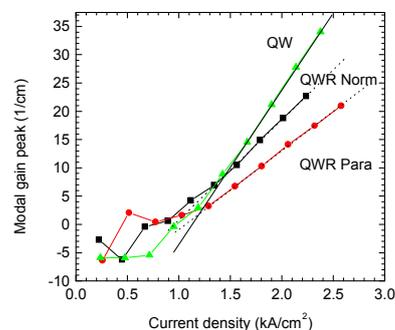
**Fig.2** Modal gain peak as a function of current density and stripe direction for (775) QWR. Data for a (100) quantum well lasers simultaneously grown are shown.
